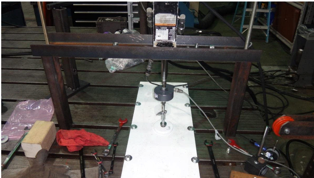
Figure 2.4.4: Tensile Individual Magnet Test Setup-Overall View
