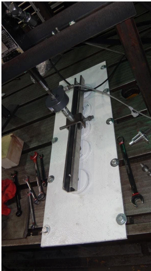
Figure 2.4.6: Tensile Uniaxial Magnemount Test Setup-Typical
